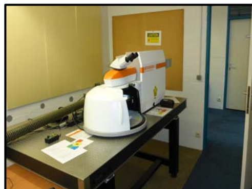
Figure 38: the ULg micro-spectroscopy labs: micro-FTIR spectrometer with Bruker Hyperion 2000 (left) and InVia Renishaw confocal micro-Raman spectrometer (right) equipped with 3 lasers (514, 632 and 785 nm).
