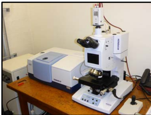
Figure 38: the ULg micro-spectroscopy labs: micro-FTIR spectrometer with Bruker Hyperion 2000 (left) and InVia Renishaw confocal micro-Raman spectrometer (right) equipped with 3 lasers (514, 632 and 785 nm).
